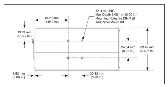
Figure C-1. Back View of the CVS-1450 Series with Dimensions
